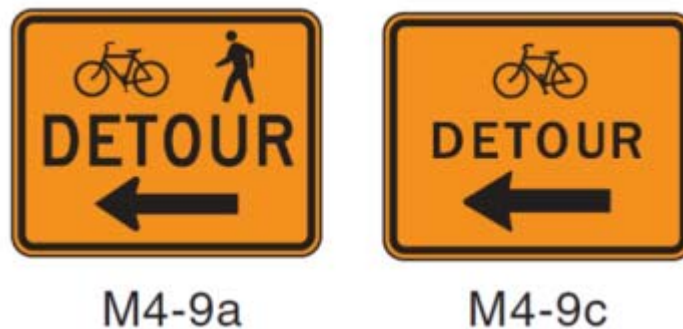
Figure 14-53 Bicycle Facility DETOUR Signs
