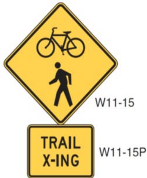
Figure 14-44 TRAIL CROSSING Assembly
