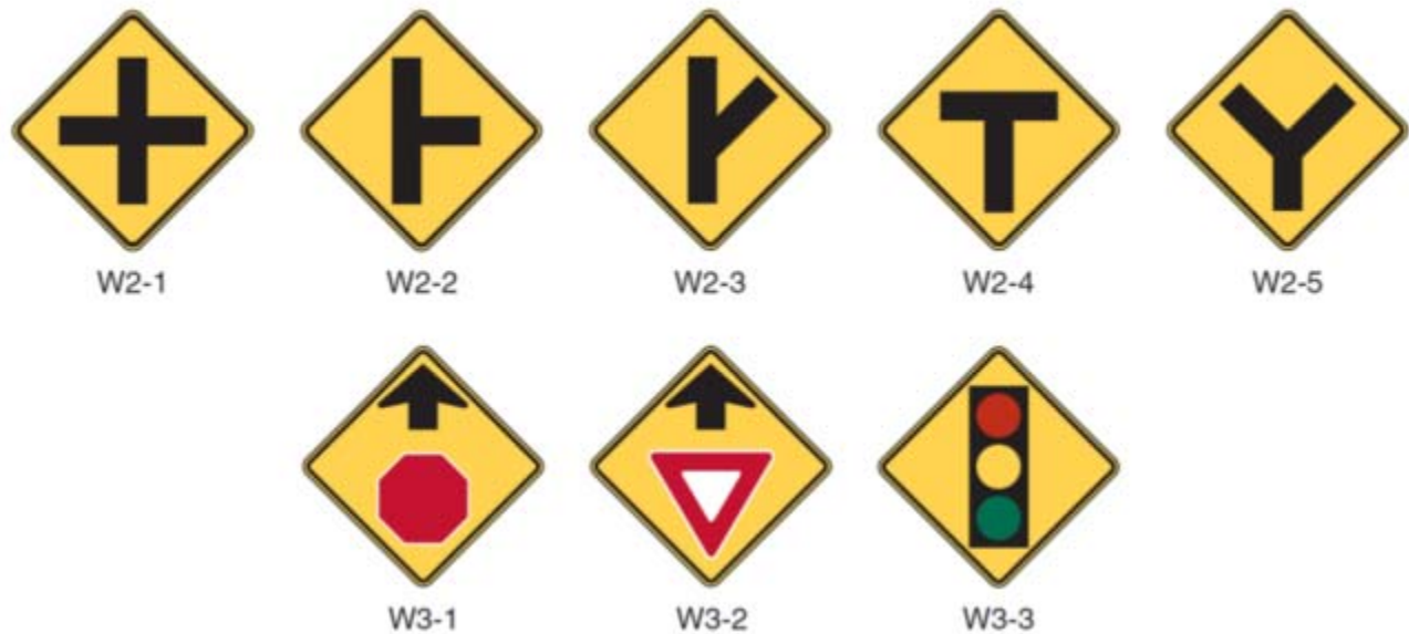
Figure 14-43 INTERSECTION WARNING (W2 Series) and ADVANCE WARNING SIGNS (W3 Series) Signs
