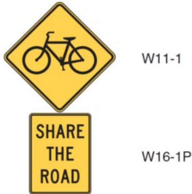
Figure 14-6 SHARE THE ROAD Sign Assembly
